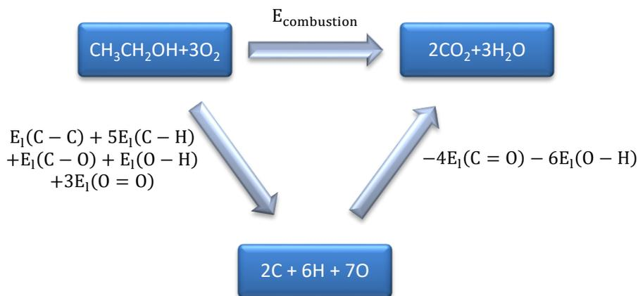
$$E_{\text{combustion}} = E_l(\text{C}-\text{C}) + 5E_l(\text{C}-\text{H}) + E_l(\text{C}-\text{O}) + E_l(\text{O}-\text{H}) + 3E_l(\text{O}=\text{O}) - 4E_l(\text{C}=\text{O}) - 6E_l(\text{O}-\text{H})$$
